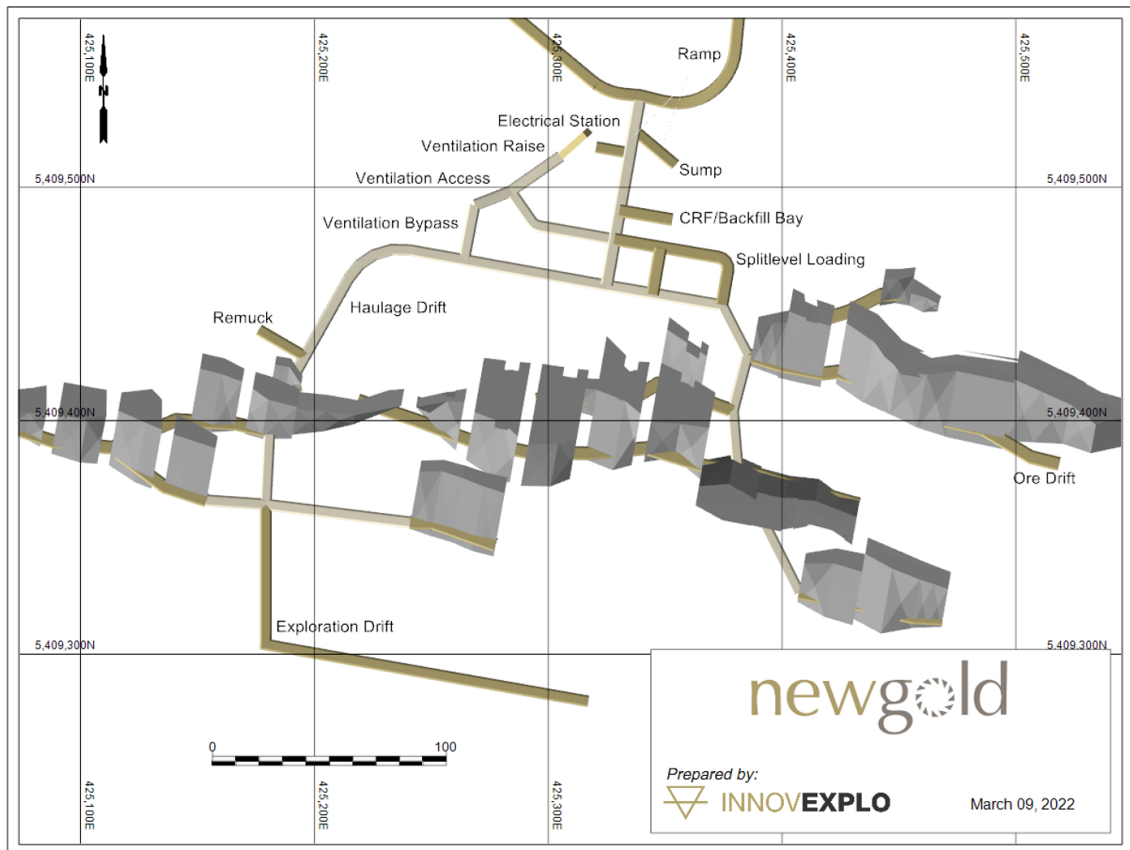
Figure 16.11 – Typical Level (ODM Main - Level UG 600)
