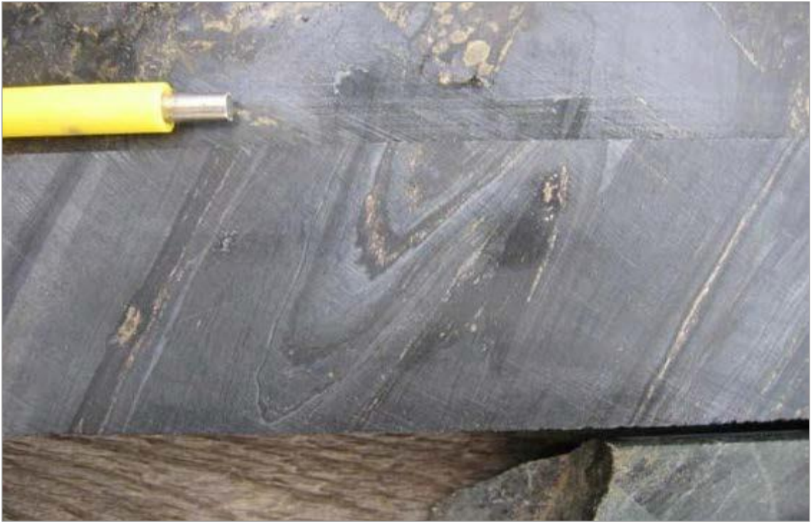
Figure 7.5 – Sulphide mineralization deformed by folding in drill core from Rainy River
